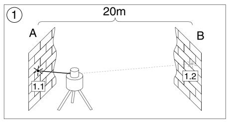
Now, place the unit near wall B with the plus X-axis pointing towards wall B. After the unit is level, mark the height of the laser beam at wall B. Turn the entire unit 180°, let it self-level and mark the center of the laser beam at wall A. The difference (h) of the marked points at wall A shows the deviation.
